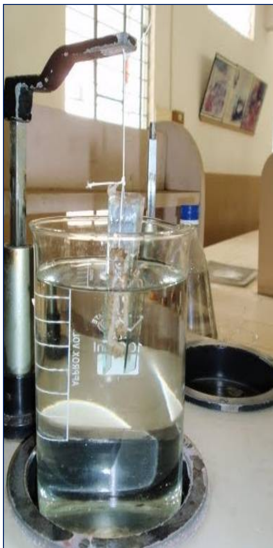
Fig. 1: The diagrammatic representation of In vitro wash off test
