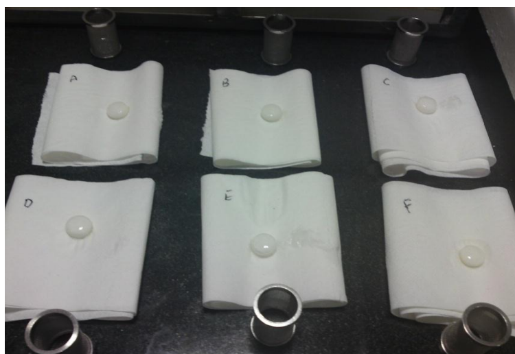
Fig. 6: Swelling phenomenon of nicotinic acid tablets
