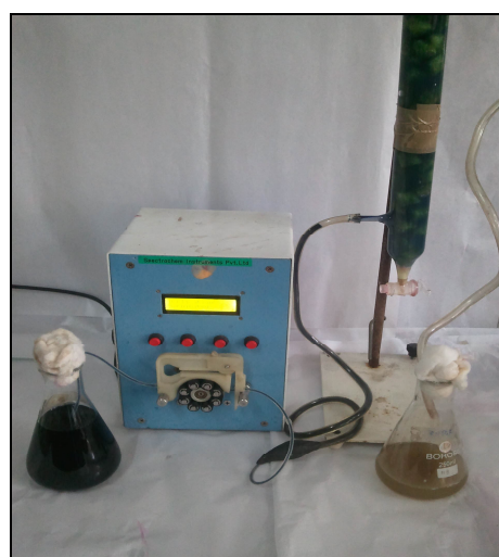
Plate. 8: Continuous degradation of Reactive Black 5 dye using PUF immobilized cells of Aeromonas punctata
