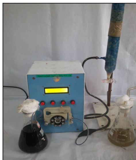
Plate. 9: Continuous degradation of Reactive Black 5 dye using Agar-Agar immobilized cells of Aeromonas punctata
