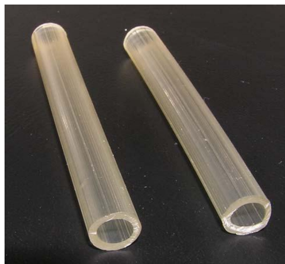
Fig. 1: Hot-melt extruded ethyl cellulose cylinders (containing 20 % dibutyl sebacate as a plasticizer)
