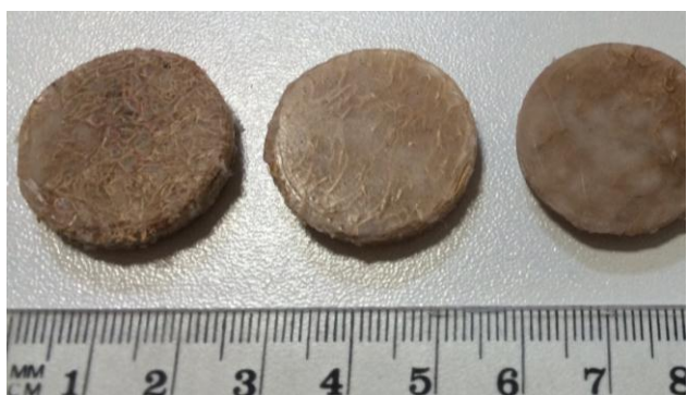
Fig. 4: Heat conductivity test samples of luffa cylindrica fibre reinforced composites
