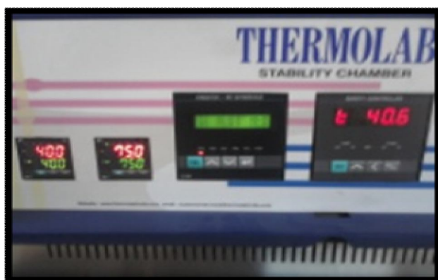
Fig. 7: Photograph showing accelerated stability condition of Stability Chamber (Thermolab®) used for studying aging behavior of optimized formulation
