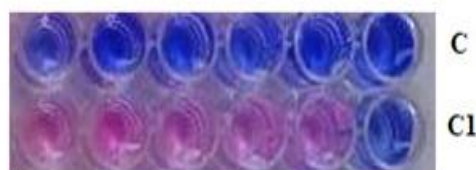
Fig. 6: Antifungal activity of the N -benzoylated tetrazolo[1,5- a ]pyrimidine-based copper(II) complex (1) against fungal strain Candida krusei by resazurin reduction assay
